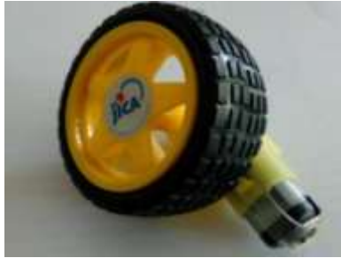
Fig. 2. DC motor and Wheel
